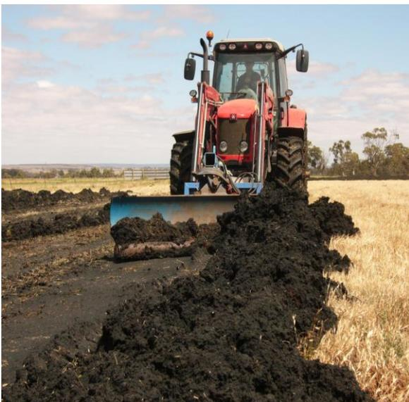
Melton RWP biosolids windrow tractor with modified grader blade.
