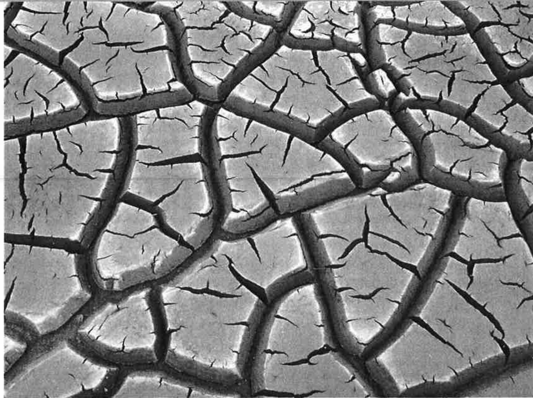
Close-up of sludge on a Deskins quick-dry filter belt.
