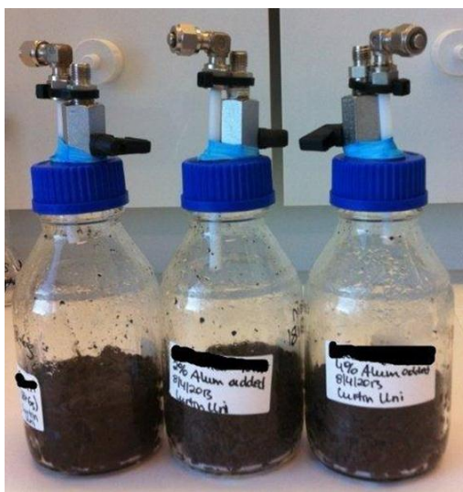
Figure 3. Lab dewatered cake samples in 500 mL Schott bottles with modified lids for analysis by dynamic olfactometry.
