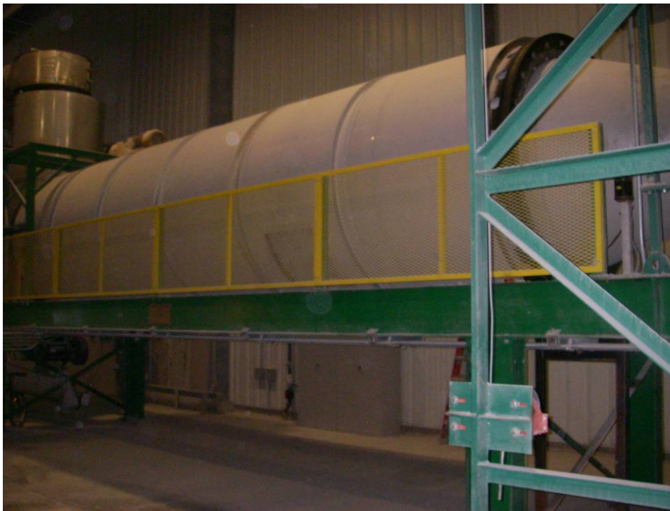
Figure 5. Dryer for Biosolids-CKD Mixture
