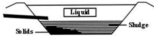
Figure 2 - Diagram of a typical Facultative Lagoon
